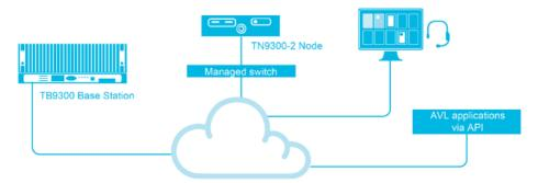
Note: The TN9300-2 node is not required if RF dispatch radio operation is the only control required with a TB9300 DMR Tier 2 base station.
